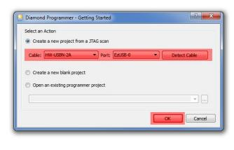
• The Lattice Diamond Programmer scan automatically the Lattice Component.
